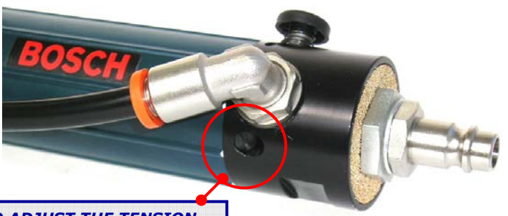
USE THIS SCREW TO ADJUST THE TENSION FORCE VALUE
